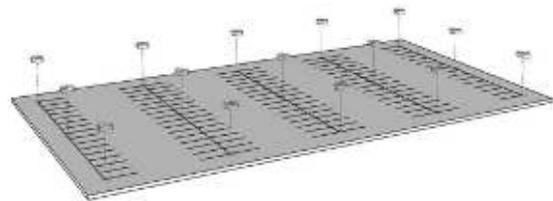
**Figure 2** Perspective view of the scale model parking lot. The observer's viewing location was from the corner at the lower left. Also shown are the locations of the LED luminaires used to illuminate the scene
