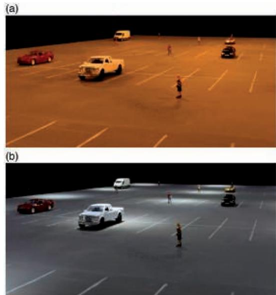
**Figure 5** (a) View of parking lot under uniform (2:1 maximum : minimum uniformity ratio), 2850 K illumination. (b) View of parking lot under non-uniform (15:1 uniformity ratio), 5800 K illumination
