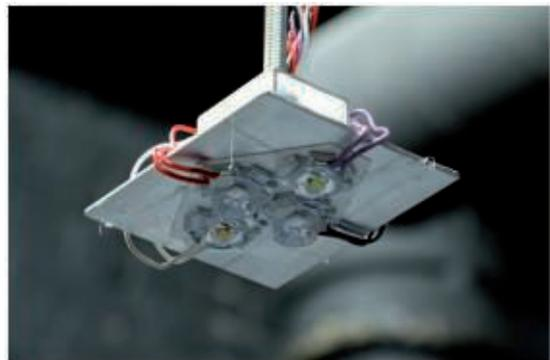
**Figure 3** Photograph of an LED luminaire used to illuminate the parking lot scene
