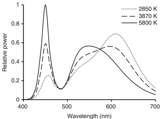
**Figure 4** Spectral power distributions for each of the correlated colour temperatures used in the experiments, scaled to equal light output
